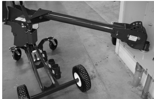
Up Pull using 45° horizontal pivot feature and one boom tube
