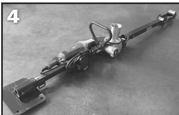
4 Cable puller shown unfolded and pinned.
