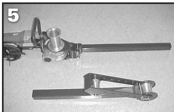
5 In order to set-up the adjustable tube in the correct direction for the pull, unpin and remove the adjustable tube from the pivot tube.
