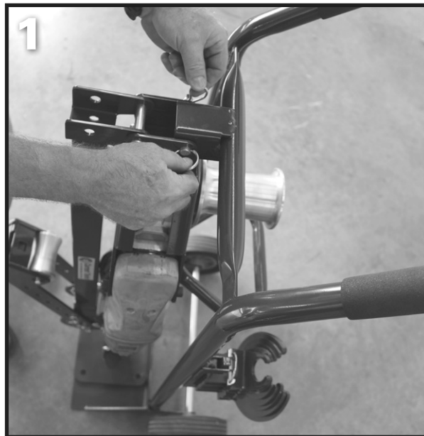
1 Remove the transport pin to release the cable puller from the mobile cart.
