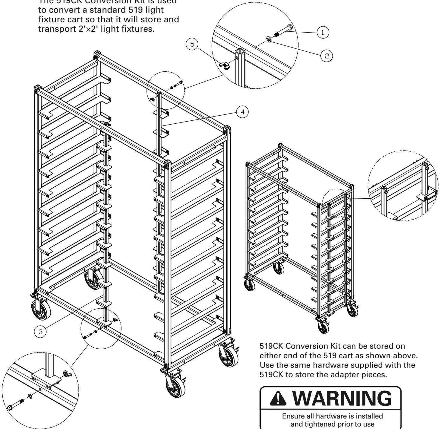
519CK Conversion Kit can be stored on either end of the 519 cart as shown above. Use the same hardware supplied with the 519CK to store the adapter pieces.
