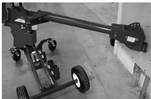
Up Pull using 45° horizontal pivot feature and one boom tube
