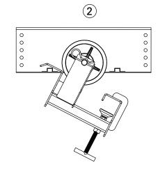
NOTE: The Speed Mount Tray Roller must be installed in the tray so that the direction of the pull goes from the clamp side of the tray roller towards the front side (See instruction #3).
