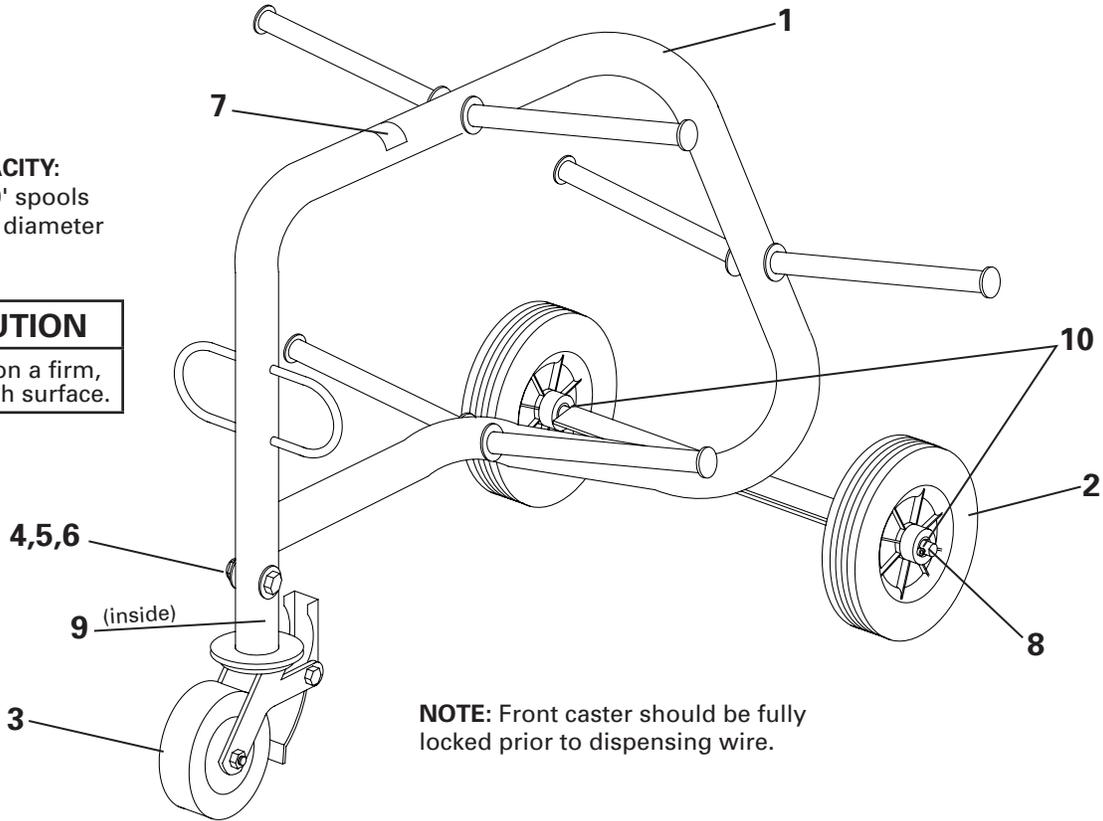
**NOTE:** Front caster should be fully locked prior to dispensing wire.
