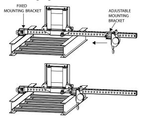
4. Tighten the thumb screw on the adjustable mounting bracket. Release the ratchet and pull the strap underneath the cable tray. Attach the strap end to the mounting loop on the fixed mounting bracket and use the ratchet to tighten the strap.
