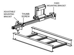
2. Place the Cross Cable Tray Roller onto the cable tray, ensuring that both mounting brackets are on the outside of the cable tray rails.
