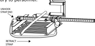
3. Loosen the thumb screw on the adjustable mounting bracket and slide the bracket away from the cable tray rail.
