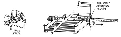
4. Lift and slide the Cross Cable Tray Roller towards the operator, allowing the cable or wire bundle to fall into the tray.
