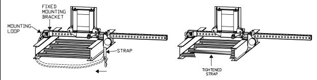
5. Adjust the position of the 4 sided rollers by pulling the spring loaded plunger pin out and sliding the roller frame to the desired position. Ensure that the pin engages one of the holes in the perforated tube when released. You are now able to pull cable.
