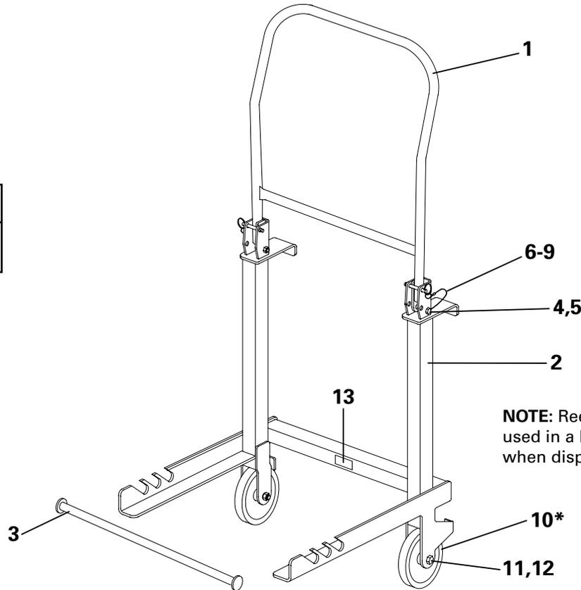
**NOTE:** Reel Dolly must be used in a horizontal position when dispensing wire.
