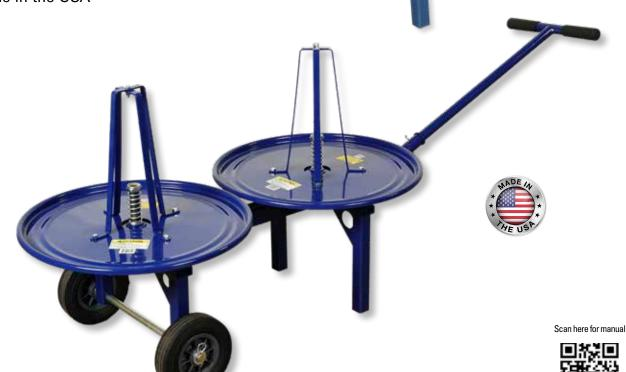
Catalog Number Description Weight 509DMC **Dual Mobile Armored Cable Dispenser** 48 lbs. UPC 811993027222 Transport Capacity – up to 2 coils armored cable weighing up to 50 lbs. per turntable (100 lbs. total) Dispensing Capacity per turntable -250' coil of 14/2, 14/3, 12/2 or 12/3 armored cable OR 250' coil of unboxed Romex®\* (50 lbs. MAX)
