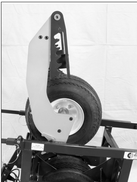
Upper drive arms raised and shown latched into open position
