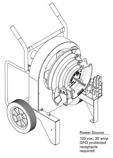
Only one shoe and roller support needed to bend 1/2"-2" for each type of conduit.
