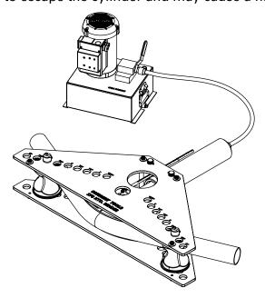
6. When the desired degree of bend is complete, rotate the pump valve lever to the open position to release the hydraulic pressure and the hydraulic cylinder will retract. Move the conduit to the next bending position.
