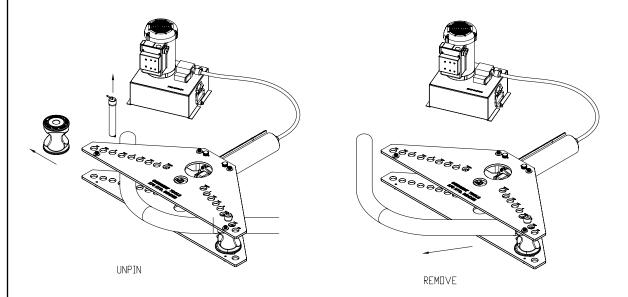
NOTE: To facililate easy removal of bent conduit, slightly retract the cylinder and remove one conduit support from the bending frame. Then operate the pump to advance the cylinder until the conduit releases from the shoe.
