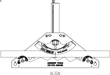
3. Rotate the pump valve lever to the closed position and activate the hydraulic pump until the shoe contacts the conduit and the conduit is tight against the conduit supports. DO NOT BEGIN BEND.
