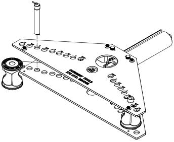
5. Turn the conduit support so that the correct side for the size conduit you are bending is facing the hydraulic cylinder.
