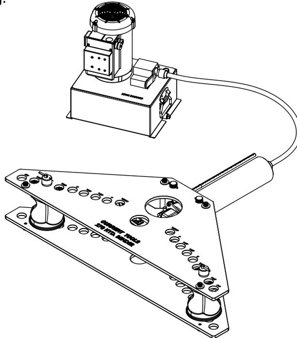
7. Adjust the gauge rod on the cylinder such that gauge reads zero when the cylinder is fully retracted. NOTE: To adjust gauge rod, loosen gauge rod adjusting nuts and adjust rod such that zero (Ø) is flush with the top of the cylinder block.
