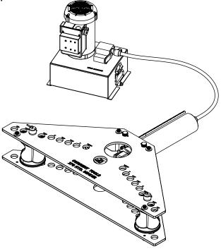
7. Adjust the gauge rod on the cylinder such that gauge reads zero when the cylinder is fully retracted.
