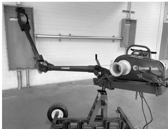
Down Pull using elbow unit and nose unit with RotaBoom™ feature
